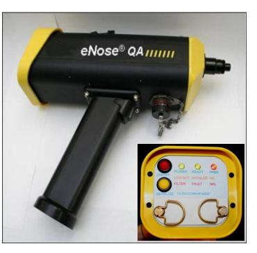
in 3 seconds after pulling the trigger. Tens of thousands of tests are made per year. The system provides ready, alarm, and self-test status via indicators (LED, LCD) and alarms.
