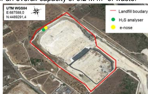
Figure 1b: sanitary landfill and monitoring points
