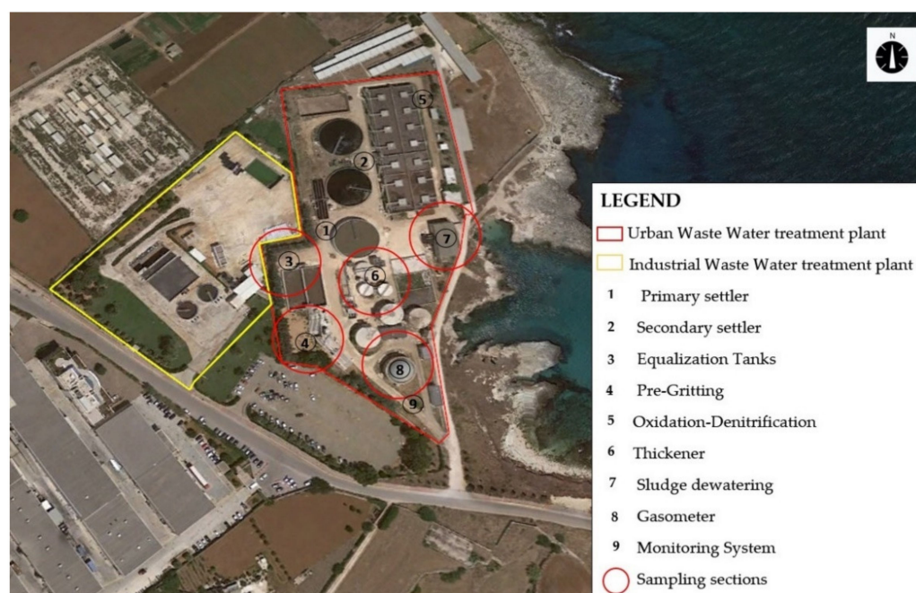
Figure 1. WWTP of Monopoli, indicating the sampling points.
